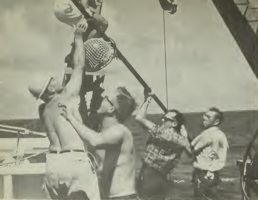
TOUGH TEST —Glass sphere is secured on carriage for a trip into the sea.
